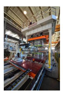
Fully automatic Cannon preformers for Carbon fibres are characterised by fast cycle times and wide platens sizes, suitable for the largest automotive Composite parts. [Square and vertical pictures available]
