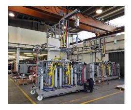
Cannon G-System - dispenser for two-component adhesives used for the largest wind blades.
