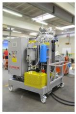
The Cannon degassing unit used to avoid the formation of air bubbles in the wind blades.
