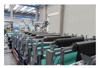
Dedicated Carbon unrolling dispensers are designed by Cannon according to each moulding project and preform characteristic.
