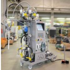
The Cannon DX Epoxy resin dispenser for the infusion of formulations in the largest wind blades.
