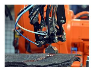
Liquid Lay Down or Spray Lay Down dispensing technologies can be utilised with multicomponent Epoxy and Polyurethane formulations
